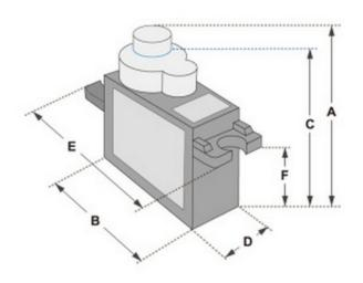
Position "0" (1.5 ms pulse) is middle, "90" (~2ms pulse) is middle, is all the way to the right, "-90" (~1ms pulse) is all the way to the left.
